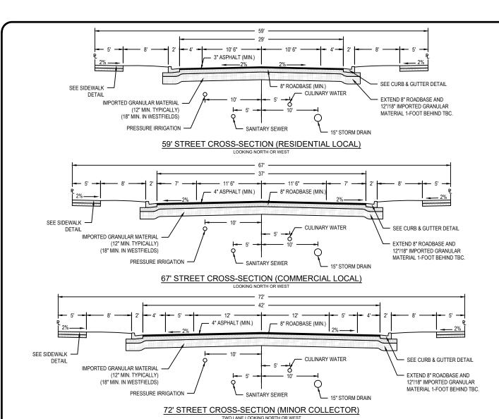
42' 12' 4" ASPHALT (MIN.) 8" ROADBASE (MIN. SEE SIDEWALK **CULINARY WATER** SEE CURB & GUTTER DETAIL DETAIL IMPORTED GRANULAR MATERIAL (12" MIN. TYPICALLY) EXTEND 8" ROADBASE AND 12"/18" IMPORTED GRANULAR (18" MIN. IN WESTFIELDS) MATERIAL 1-FOOT BEHIND TBC. PRESSURE IRRIGATION SANITARY SEWER - 15" STORM DRAIN
