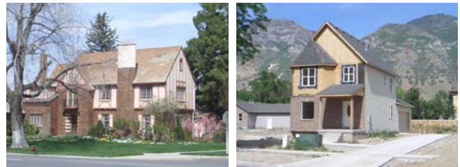
Left: materials on this house are appropriate and consistent on all sides. Right: the lack of brick on the side of the house detracts from its character.
